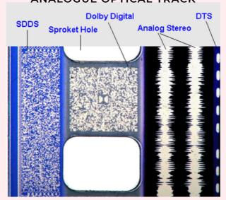
THE TRACK ON THE INSIDE OF THE PERFORATIONS IS A VARIABLE AREA DOLBY SR (SPECTRAL RECORDING) ANALOGUE OPTICAL TRACK. THE ANALOGUE OPTICAL TRACK WAS THE PRINCIPAL WAY TO PLAY BACK FILM SOUND FROM THE 1920S TO THE 1990S. AS DESCRIBED IN THE SOUND HEAD SECTION, VARIATIONS IN LIGHT FROM THE ANALOGUE OPTICAL TRACK ARE PICKED UP AND CONVERTED
